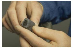
1. Cut off the desired amount to be used. Peel off protective wrap.
