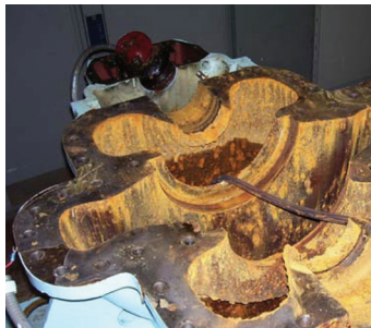
Before: cavitation, erosion/corrosion
