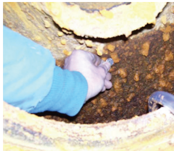
Close up: cavitation, erosion/corrosion
