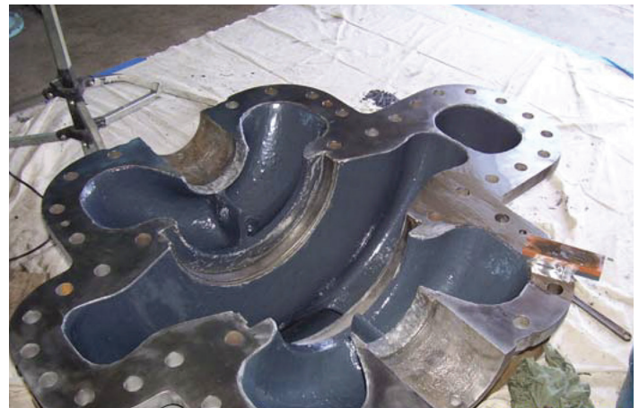
After: blasting, metal filler, 2 top coats
