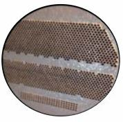
Heat Exchangers, Chillers and Condensers are constructed of bundles of copper tubes held together by tube plates, all of which are contained in a solid metallic cylinder. If these units are left unattended, the corrosion would completely destroy the tube plate as seen in the photo. USI has the required coatings that can withstand the aggressive operating environment. These coatings will give you the repair, protection and upgrade that you are looking for.
