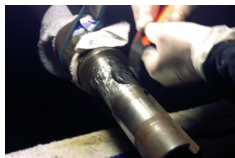
USI Metal Repair EG was properly mixed
