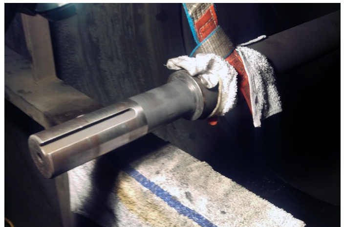
This shaft was allowed to finish curing and was back in service within 48 hours
