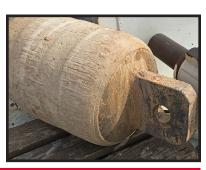
PHOTO: Bore-head with Stop It® Boreshield™ Minimal Damage after 4 sequential pulls of ~1000 FT, preserving the integrity of the weld.
