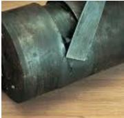
To apply HAR you press material thoroughly into substrate and insure a completely wetted out surface. HAR may be over coated with other DUROMAR materials such as EAC or EP for enhanced smoothness or increased chemical resistance. Over coating may begin as soon as the first coat is firm enough to accept a second coat. In high humidity or cold temperatures, a blush may develop which should first be wiped down with clean water.
